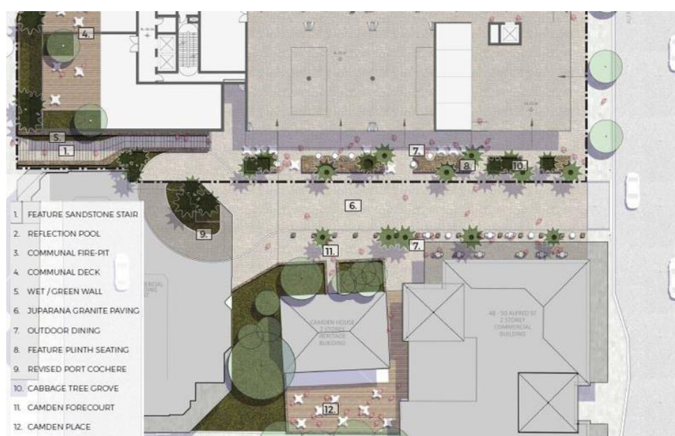
Figure 30 Proposed indicative design of the through-site link
